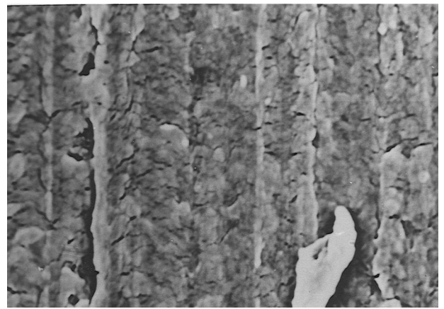
Figure 20 Scanning electron micrograph of establishment of the transfer film at 700\times for UHMWPE (same conditions as Fig. 19).
